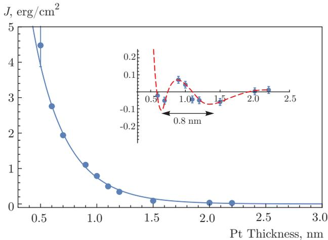
**Fig. 1.** Interlayer exchange coupling strength vs. thickness of Pt spacer layer. The line is a fit using an exponential fit derived from free energy of the Landau theory of phase transitions, yielding  $\xi = 0.31 \pm 0.1$  nm. Inset shows the residuals to the fit, the dashed line is a guide for the eye. Reprinted with permission from Omelchenko Appl. Phys. Lett. **113**, 142401 (2018). Copyright 2018, American Institute of Physics
