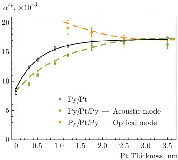
**Fig. 3.** Damping with increasing thickness of Pt for the  $\text{Py}/\text{Pt}(d_{\text{Pt}})$ , the acoustic mode of  $\text{Py}/\text{Pt}(d_{\text{Pt}})/\text{Py}$  and optical mode of  $\text{Py}/\text{Pt}(d_{\text{Pt}})/\text{Py}$ . The solid line is a fit to the  $\text{Py}/\text{Pt}(d_{\text{Pt}})$  data using the conventional spin-pumping model. The dashed lines are simulations of the damping for the acoustic and optical modes by the process described in Omelchenko et al. [8]
