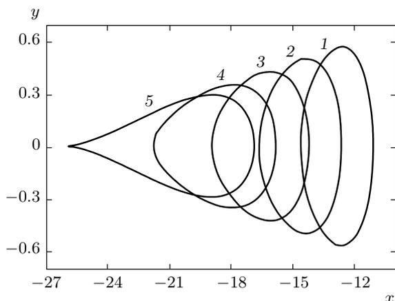
**Fig. 1.** Evolution of the bubble boundary corresponding to exact solutions (27), (29)–(31), where  $s = 1$ ,  $k = -0.02$ ,  $t_1 = -11$ ,  $\alpha_1 = 0$ , and the upper sign “+” is taken. The boundary shape is shown for the successive instants  $t = 0$ ,  $t = 0.5$ ,  $t = 0.9$ ,  $t = 1.2$ , and  $t = t_c \approx 1.341$
