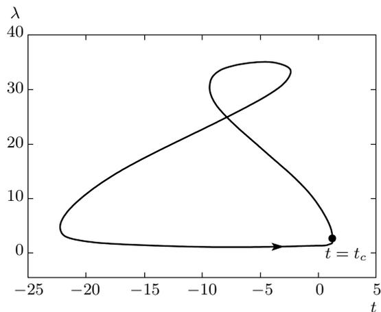
**Fig. 2.** Time dependence of the second harmonic amplitude  $\lambda$  for  $s = 1$ ,  $k = -0.02$ , and  $t_1 = -11$  described by Eq. (31). The instant of cusp formation corresponds to the marked point  $t = t_c \approx 1.341$ ; the motion to this point occurs in the counterclockwise direction
