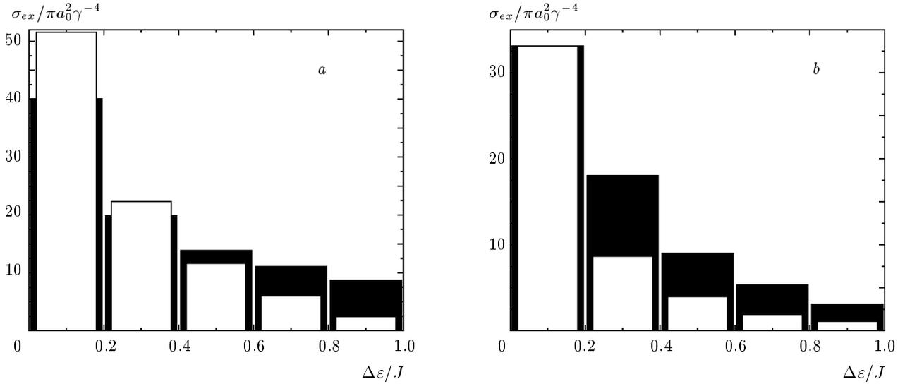
**Fig. 4.** Excitation cross sections of a Rydberg atom by electron impact at the relative collision energies  $E/J = 1.2$  (a) and  $E/J = 5$  (b); black histograms correspond to numerical evaluations and white histograms relate to the Thomson model
