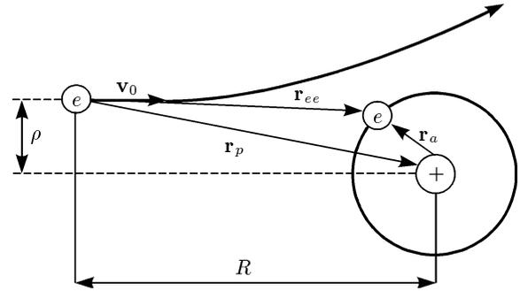
Fig. 1. Positions of the Coulomb center, the incident electron, and the bound electron in a collision of an electron and a Rydberg atom
