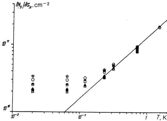
FIG. 8. Temperature dependences of the reciprocal of the maximum value of the derivative  $\partial\sigma_{xy}/\partial N_s$ : (○)  $i \approx 3.5$ , (\*)  $i \approx 2.5$ , sample No. 3,  $H = 16$  T; (□)  $i \approx 3.5$ , (△)  $i \approx 2.5$ , sample No. 2,  $H = 16$  T; (▲)  $i \approx 3.5$ , sample No. 2,  $H = 10$  T; (☆)  $i \approx 3.5$ , (■)  $i \approx 2.5$ , sample No. 1,  $H = 14$  T.
