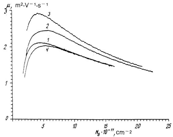
FIG. 2. Electron mobility in silicon MOS transistors plotted as a function of the electron density at  $T = 1.5 \text{ K}$ . The numbers alongside the curves are the serial numbers of samples.
