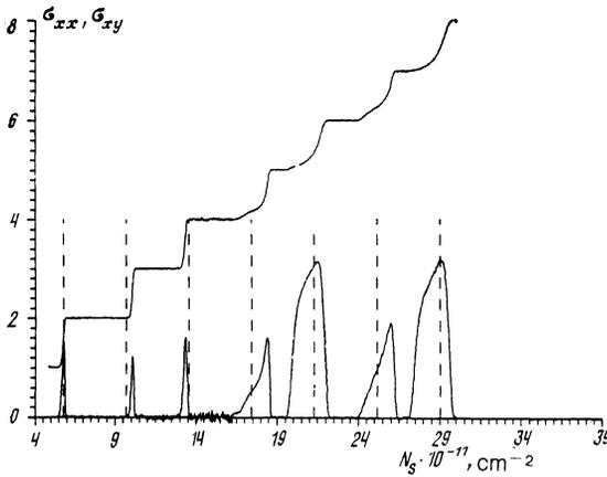
FIG. 3. Dependences of  $\sigma_{xx}$  and  $\sigma_{xy}$  on the electron density in sample No. 1. The ordinate is in units of  $e^2/h$  and the values of  $\sigma_{xx}$  are increased by a factor of 10. The dashed vertical lines represent the position of the half-integral occupancy factors.  $H = 16$  T,  $T \approx 20$  mK.
