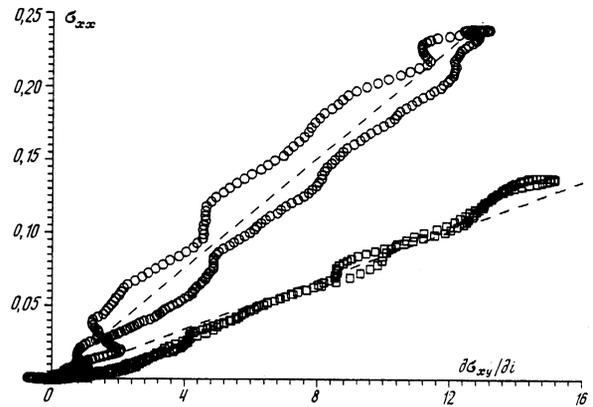
FIG. 10. Conductivity  $\sigma_{xx}$  plotted as a function of the derivative  $\partial\sigma_{xy}/\partial i$  for two  $\sigma_{xx}$  peaks: (○)  $i \approx 3.5$ , (□)  $i \approx 2.5$ , sample No. 3,  $H = 16$  T,  $T \approx 20$  mK.
