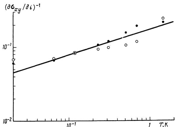
FIG. 13. Temperature dependence of the fraction of delocalized states  $\alpha_0$  at a quantum level:  $\circ$ )  $i \approx 1.5$ ,  $\bullet$ )  $i \approx 3.5$ ; sample MP2.
