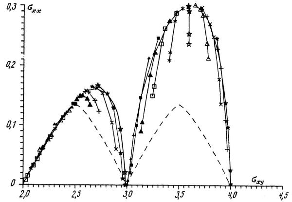
FIG. 5. Flow line pattern for sample No. 3. The dashed curve represents the results of a symmetric reflection and translation of a part of a separatrix in a segment  $2 \leq (h/e^2)\sigma_{xy} \leq 2.5$ . The axes are plotted in units of  $e^2/h$ .
