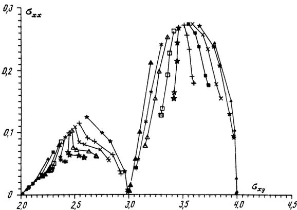
FIG. 7. Flow line pattern for sample No. 2. The saddle point is plotted for the peak  $\sigma_{xx}$  corresponding to  $i = 2.5$  and it is shifted to the left relative to the half-integral value of  $(h/e^2)\sigma_{xy}$ . The ordinate of the saddle point is considerably less than for the other silicon MOS transistors.
