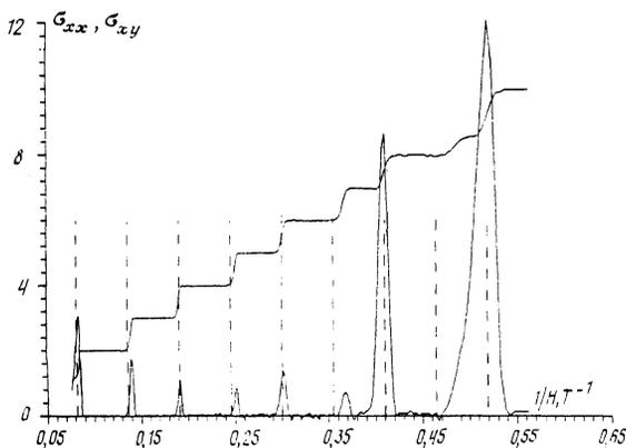
FIG. 4. Conductivities  $\sigma_{xx}$  and  $\sigma_{xy}$  of sample MP2 plotted as a function of the reciprocal of the applied magnetic field.  $T \approx 20$  mK; the values of  $\sigma_{xx}$  are increased by a factor of 100. The dashed lines represent, as in Fig. 3, the half-integral values of the occupancy factor.
