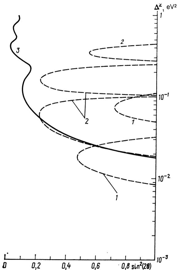
FIG. 2. Bounds on the neutrino oscillation parameters. 1—from this work; 2—from this work plus Ref. 2; 3—from Ref. 4. The confidence level for all the curves was 90%.
