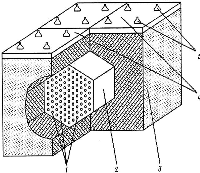
FIG. 1. Neutrino detector. 1— $^3\text{He}$  proportional neutrino counters; 2—detector; 3—shielding made of borated polyethylene; 4—films for active shielding from cosmic-ray mesons; 5—FEU-125 photomultiplier.
