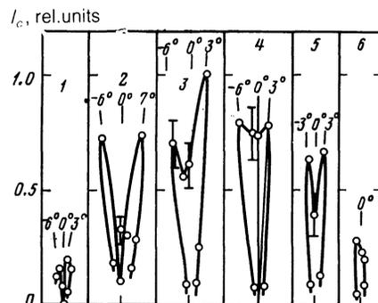
FIG. 3. Ion current reaching the collectors at various moments in time after a giant laser radiation pulse: 1)  $t = 0.6 \mu\text{s}$ ; 2)  $0.9 \mu\text{s}$ ; 3)  $1.1 \mu\text{s}$ ; 4)  $1.2 \mu\text{s}$ ; 5)  $1.9 \mu\text{s}$ ; 6)  $2.7 \mu\text{s}$ . These results were obtained for a carbon target;  $B = 0.2 \text{ T}$ ,  $L = 5 \text{ cm}$ ,  $\Phi \sim 6 \times 10^9 \text{ W/cm}^2$ .
