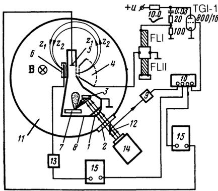
FIG. 2. Principal components of the apparatus: 1) lens; 2) entry window; 3) mirror; 4) electrode; 5), 6) collectors; 7) target; 8) casing; 9) triggering unit; 10) delay and synchronization unit; 11) vacuum chamber; 12) beam splitter; 13) fast amplifier; 14) CO<sub>2</sub> laser; 15) S8-2 oscilloscope.
