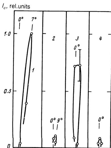
FIG. 5. Ion current reaching the collectors recorded at different moments after the formation of a plasma: 1)  $t = 1.1 \mu\text{s}$ ; 2)  $2.0 \mu\text{s}$ ; 3)  $2.3 \mu\text{s}$ ; 4)  $3.0 \mu\text{s}$ . The target was carbon;  $B = 0.5$  T;  $L = 6.5$  cm;  $\Phi \sim 4 \times 10^9$  W/cm<sup>2</sup>.
