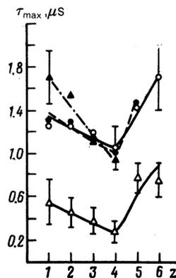
FIG. 8. Expansion time from the target to the region of analysis of the maxima of the current representing ions with different charges.  $B = 0.2$  T,  $L = 5$  cm,  $\varphi = -3^\circ$ ; ( $\Delta$ )  $\Phi \sim 3 \times 10^{10}$  W/cm<sup>2</sup>; ( $\circ$ )  $\Phi \sim 6 \times 10^9$  W/cm<sup>2</sup>; ( $\bullet$ )  $\Phi \sim 4 \times 10^9$  W/cm<sup>2</sup>; ( $\blacktriangle$ )  $\Phi \sim 10^9$  W/cm<sup>2</sup>.
