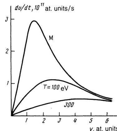
FIG. 1. The acceleration  $dv/dt$  as a function of the velocity  $v$  of the  $\alpha\mu$  ion at plasma temperatures of 100 and 300 eV. The curve marked  $M$  corresponds to the molecular medium.
