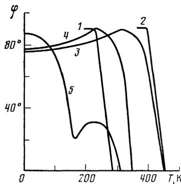
FIG. 8. Temperature dependence of the angle between the easy axis and the [001] axis for hexagonal  $\text{Nd}_2\text{Co}_7$  (1),  $\text{Tb}_2\text{Co}_7$  (2), and rhombohedral quasibinary  $(\text{Tb}_{1-x}\text{Y}_x)_2\text{Co}_7$  with  $x = 0$  (3), 0.2 (4), and 0.4 (5).
