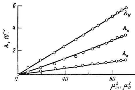
FIG. 3. Spontaneous linear ( $\lambda_a, \lambda_c$ ) and volume ( $\lambda_V$ ) magnetostriction deformations in  $Y_2Co_7$ , as functions of the square of the molecular magnetic moment  $\mu_m$ .
