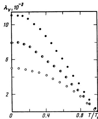
FIG. 7. Temperature dependence of the spontaneous volume magnetostriction  $\lambda_V$  for  $\text{Nd}_2\text{Co}_7$  (○),  $\text{Gd}_2\text{Co}_7$  (●), and  $\text{Tb}_2\text{Co}_7$  (●).
