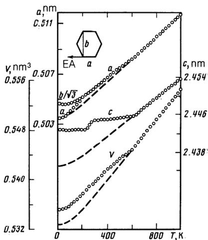
FIG. 5. Temperature dependence of  $a, c, V$ , and the rhombic distortions in  $Nd_2Co_7$ .
