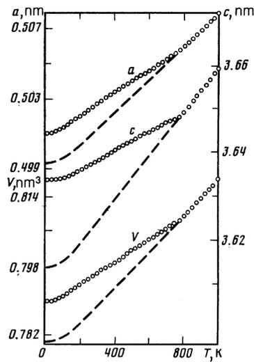
FIG. 4. Temperature dependence of the lattice parameters  $a, c$  and unit cell volume  $V$  for  $Gd_2Co_7$ .
