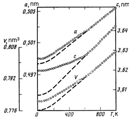
FIG. 2. Temperature dependence of the lattice parameters  $a$ ,  $c$  and unit volume  $V$  for rhombohedral  $Y_2Co_7$ .
