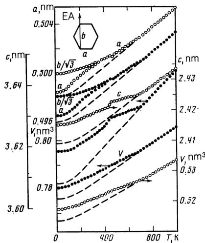
FIG. 6. Temperature dependence of  $a$ ,  $c$ ,  $V$ , and the rhombic distortions for hexagonal (○) and rhombohedral (●)  $\text{Tb}_2\text{Co}_7$ .
