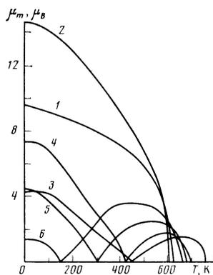
FIG. 1. Temperature behavior of the molecular magnetic moments  $\mu_m$  (divided by the Bohr magneton  $\mu_B$ ) for  $Y_2Co_7$  (1),  $Nd_2Co_7$  (2),  $Gd_2Co_7$  (3),  $Tb_2Co_7$  (4),  $(Tb_{0.8}Y_{0.2})_2Co_7$  (5),  $(Tb_{0.6}Y_{0.4})_2Co_7$  (6).
