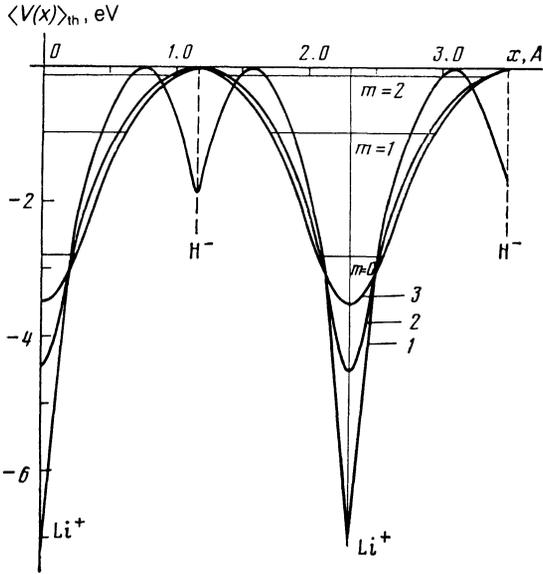
FIG. 1. Structure of electron interaction potentials in (111) planes of an LiH crystal in the "frozen" case when the mean-square displacements of the ions  $u_1$  and  $u_2$  are zero (curve 1) and in the case of phonon flattening at  $T = 0$  K and  $T = 300$  K (curves 2 and 3, respectively). In the last case the levels of the channeled electrons are shown for  $E = 20$  MeV.
