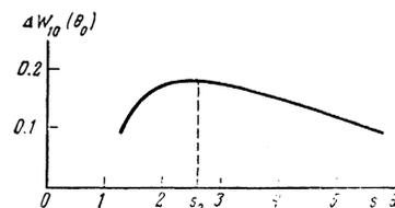
FIG. 2. Population inversion  $\Delta W_{10}(\theta_0)$  between the two lowest energy levels calculated for the optimal angle  $\theta_0$  of entry into a crystal as a function of the parameter  $s$ .
