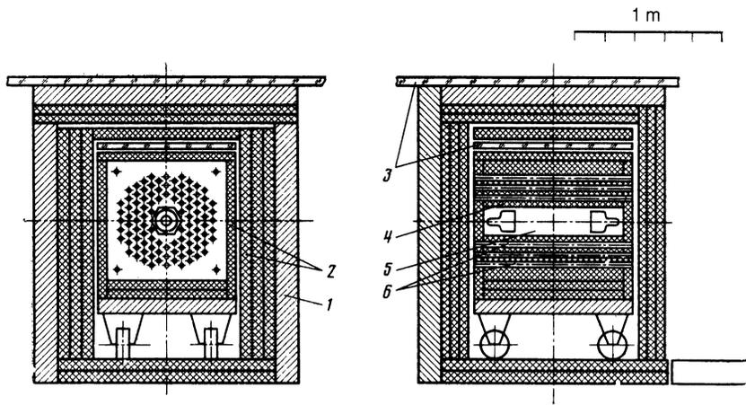
FIG. 1. External view of the detector; 1—gamma ray field (copper), 2—neutron shield (borated polyethylene), 3—active shield, 4—moderating target (plexiglass), 5—scintillation section, 6— $^3\text{He}$  neutron counters.
