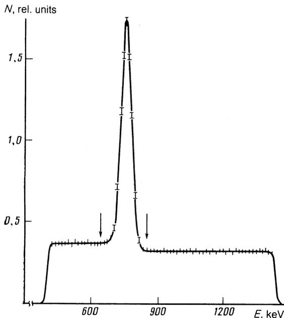
FIG. 2. Differential pulse-height spectrum produced by IND. Arrows define the neutron detection window.
