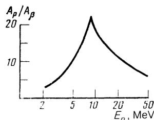
FIG. 1. Ratio of average amplitudes of signals from protons of energy  $E$  and from electrons of energy  $\sim 1$  MeV perpendicularly incident on a scintillator 1 mm thick.
