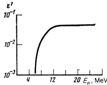
FIG. 3. Probability of recording a proton by one counter vs the proton energy.
