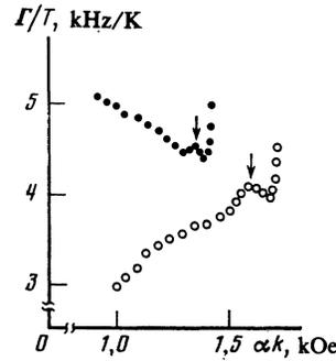
FIG. 1. Behavior of the NSW relaxation in CsMnF<sub>3</sub> in the coordinates ( $\Gamma/Tak$ ) at a pump frequency  $\nu_p = 1022$  MHz at two temperatures: 4.23 K (filled dots) and 3.03 K (open dots). The arrows indicate the positions of the transverse magnon-phonon peak.
