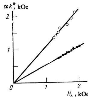
FIG. 2. Temperature dependence of the positions of the transverse (open dots,  $\nu_p = 1022$  MHz) and longitudinal (filled dots,  $\nu_p = 775$  MHz) magnon-phonon peaks in the NSW relaxation of CsMnF<sub>3</sub>, in the coordinates  $(\alpha k^*, H_\Delta \propto T^{-1/2})$ , in which the theoretical curves should be straight lines passing through the origin [Eq. (11)].
