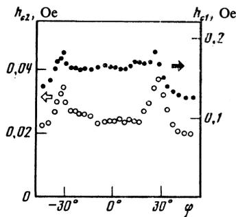
FIG. 4. Threshold fields  $h_{c1}$  and  $h_{c2}$  for the parametric excitation of NSWs in  $\text{CsMnF}_3$  versus the direction of  $\mathbf{H}$  in the basal plane of the crystal ( $\varphi = 0$  corresponds to the two-fold axis of the crystal):  $T = 1.95$  K,  $H_0 = 0.94$  kOe,  $\nu_p = 784$  MHz.
