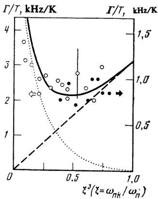
FIG. 5. Frequency dependence of the NSW relaxation for CsMnF<sub>3</sub> (open dots, left-hand scale) and CsMnCl<sub>3</sub> (filled dots, right-hand scale) in the coordinates ( $\Gamma/T, \xi^3$ ) for  $\alpha k = 1$  kOe. The dashed line is the theoretical dependence from (13), the dotted curve is the contribution to the NSW relaxation due to the ESW damping (12), and the solid curve is the sum of these curves (14);  $\xi = \omega_{nk}/\omega_n$ .
