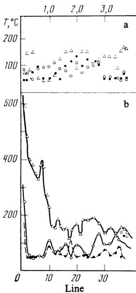
FIG. 6. Heating of the limiter during the injection of microwave power into a chamber without a plasma. Poloidal temperature profiles: a) Before the microwave pulse; b) during the microwave pulse, 85 ms after the beginning of this pulse.  $\triangle$ —First column of points, “ion side” of the limiter;  $\bullet$ —second column of points, crest of limiter;  $\circ$ —third column of points, “electron side” of limiter.
