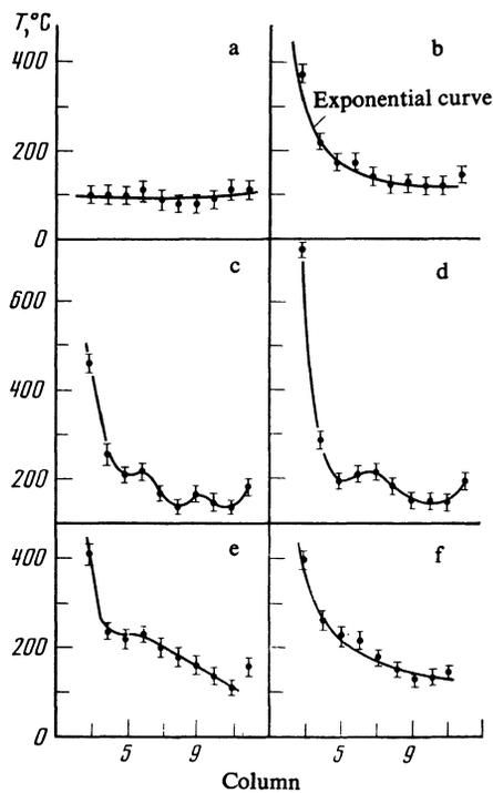
FIG. 4. Toroidal temperature profiles (averaged over lines 15–19). a) During the linear current increase; b) in the current plateau (358 ms into the discharge); c, d) during the microwave pulse (438 and 477 ms into the discharge); e) after the gyrotrons are turned off (557 ms into the discharge); f) after the discharge has ended (at 636 ms).
