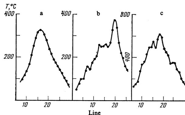
FIG. 3. Poloidal temperature profiles. a) In a discharge without disruptions, during the current plateau; b) in a discharge with a disruption, in the initial stage of the disruption; c) in a discharge without a disruption, during the current growth.
