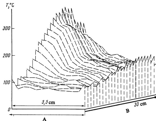
FIG. 2. Limiter temperature field during the plateau in the discharge current at 603 ms. Each curve corresponds to a single line on the screen of the heat visualizer. The hatching shows the "hottest line" (near the middle of the limiter). A) Toroidal direction; B) poloidal direction (individual lines).
