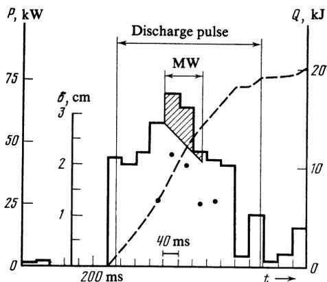
FIG. 7. Results of a calculation of the power  $P$  (solid line) dissipated at the limiter, of the decay constant  $\delta$  (●), and of the energy  $Q$  (dashed line) accumulated in the limiter for pulse No. 28565. The microwave heating power is 450 kW; there is essentially no soft x-ray emission; the plasma density is decaying. The hatching shows the additional power increase caused by the operation of the gyrotrons.
