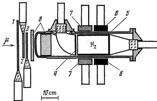
FIG. 1. Diagram of experimental apparatus: 1—guard detector; 2, 3, and 4—monitor counters; 5—cup counter enclosing the target working volume; 6 and 7— $\gamma$  and  $e$  counters with respective scintillators of NaI(Tl) and plastic; 8—absorber to slow down muons.
