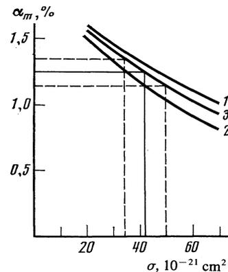
FIG. 4. The relation  $\alpha_m(\sigma)$  for the following effective masses of the molecules: curve 1— $M = m_p$ , curve 2— $M = 2m_p$ , curve 3— $M = 1.25m_p$ . On the ordinate axis we have shown the measured value of  $\alpha_i$  and on the abscissa we have shown the resulting value of  $\sigma(p\mu + H_2)$ .
