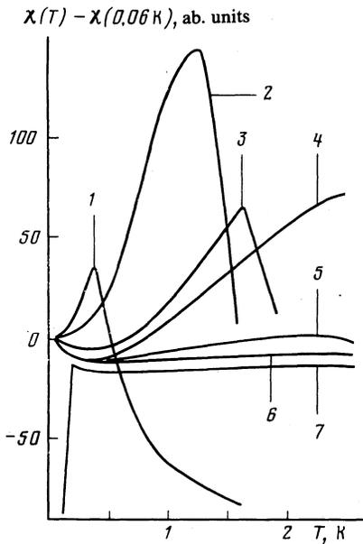
FIG. 2. Magnetic susceptibility  $\chi(T) - \chi(0.06 \text{ K})$ , ab. units for different values of  $x$  (1—0.02; 2—0.5; 3—0.6; 4—0.7; 5—0.9; 6— $\text{CeCu}_2\text{Si}_2$ , single crystal). Curve 7 corresponds to  $\chi(T)$  for polycrystalline  $\text{CeCu}_2\text{Si}_2$ .
