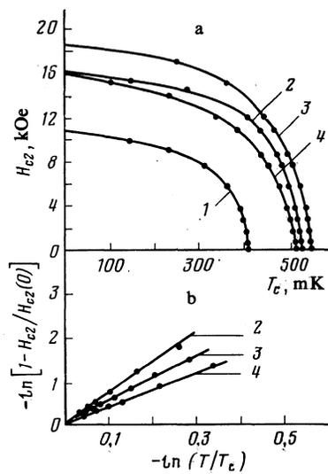
FIG. 9. Critical field  $H_{c2\parallel}(T_c)$  (a) and the function  $\ln[1 - H_{c2}/H_{c2}(0)] = -\alpha \ln(T/T_c)$  (b) for different pressures: 1—2.2 kbar; 2—3.2 kbar ( $\alpha \simeq 8$ ); 3—5 kbar ( $\alpha \simeq 6$ ); 4—12 kbar ( $\alpha \simeq 4$ ).
