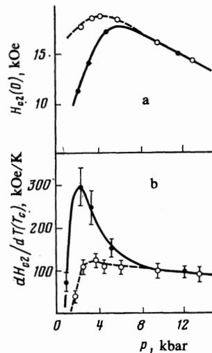
FIG. 8. Pressure dependence of the upper critical field  $H_{c2}(0)$  (a) and of the derivative  $dH_{c2}/dT(T = T_c)$  (b) for different directions of the magnetic field  $H$  and measuring current  $I$ :  $H \parallel I$  (○) and  $H \perp I$  (●).
