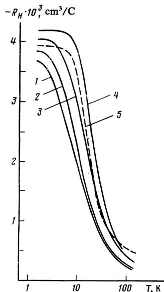
FIG. 5. Hall coefficient  $R_H$  of a  $CeCu_2Si_2$  single crystal under different pressures (1—0.25 kbar; 2—0.9 kbar; 3—4 kbar; 5—9 kbar; 5—13.5 kbar).
