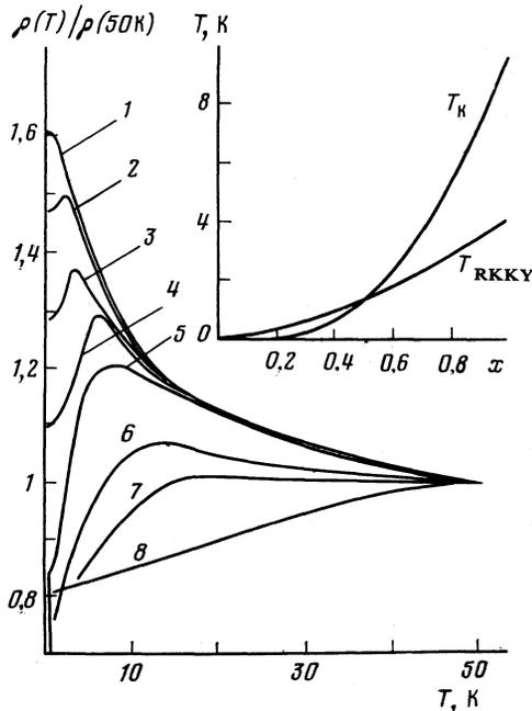
FIG. 1. Resistivity of the solid solutions Ce<sub>x</sub>La<sub>1-x</sub>Cu<sub>2</sub>Si<sub>2</sub> for different  $x$  (1—0.2; 2—0.4; 3—0.5; 4—0.7; 5—1) and CeCu<sub>2</sub>Si<sub>2</sub> under pressure (6—10 kbar; 7—16.6 kbar; 8—45 kbar).
