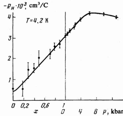
FIG. 7. Hall coefficient  $R_H$  (4.2 K) as a function of  $x$  for  $\text{Ce}_x\text{La}_{1-x}\text{Cu}_2\text{Si}_2$  and as a function of pressure  $p$  for the  $\text{CeCu}_2\text{Si}_2$  single crystal.
