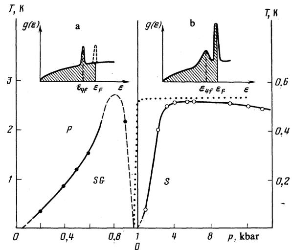
FIG. 3. Phase diagram for the magnetic and superconducting properties of the system  $\text{Ce}_x\text{La}_{1-x}\text{Cu}_2\text{Si}_2$  for  $0 < x < 1$  and  $0 < p < 13.4$  kbar (P—paramagnetic phase, SG—spin glass, S—superconducting phase). The function  $T_c(x, p)$  is shown by the points and corresponds to Steglich's data.<sup>14</sup> Insets show the density of states  $g(\epsilon)$  for  $T_K < T_{\text{RKKY}}$  (a) and  $T_K > T_{\text{RKKY}}$  (b).
