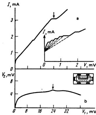
FIG. 1. a) Current-voltage characteristic of film 1. The inset shows the initial section of the CVC;  $T=1.72$  K. b) Drag-signal voltage  $V_2(V_1)$  and construction of the dc superconducting transformer. The arrows mark the step on the CVC (a) and the corresponding singularity in the drag signal  $V_2(V_1)$  (b).
