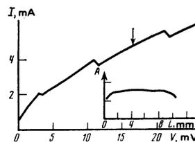
FIG. 2. Current-voltage characteristic of aluminum film at  $T=1.71$  K. The inset shows the dependence of the second-sound signal amplitude on the coordinate  $L$  along the aluminum film. The arrow indicates the region of the bias voltage on the film, at which the measurements on second-sound generation in helium were performed.
