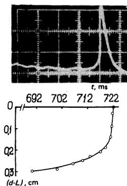
FIG. 1. Time dependence of the distance from the tip of the twin to the surface of the crystal ( $d-L$ ) juxtaposed with the oscillogram of the sound emission in the same time scale. The scale of the oscillogram along the abscissa is  $5 \mu\text{s/cm}$ .
