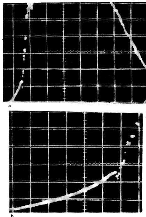
FIG. 2. Oscillogram of the signal of acoustic emission accompanying the approach of the pile up of dislocations from the interior of the crystal to the surface with its subsequent emergence to the surface: a) the minimum scale division along the abscissa is  $8 \mu\text{s}$ ; b) the minimum scale division along the abscissa is  $1.6 \mu\text{s}$ .
