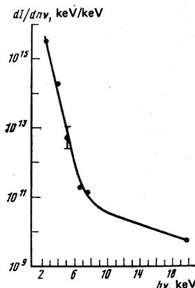
FIG. 4. Spectral distribution of intensity of  $x$  radiation of the plasma corona (aluminum target,  $E = 140 \text{ J}$ ,  $\tau = 3.0 \text{ nsec}$ ).
