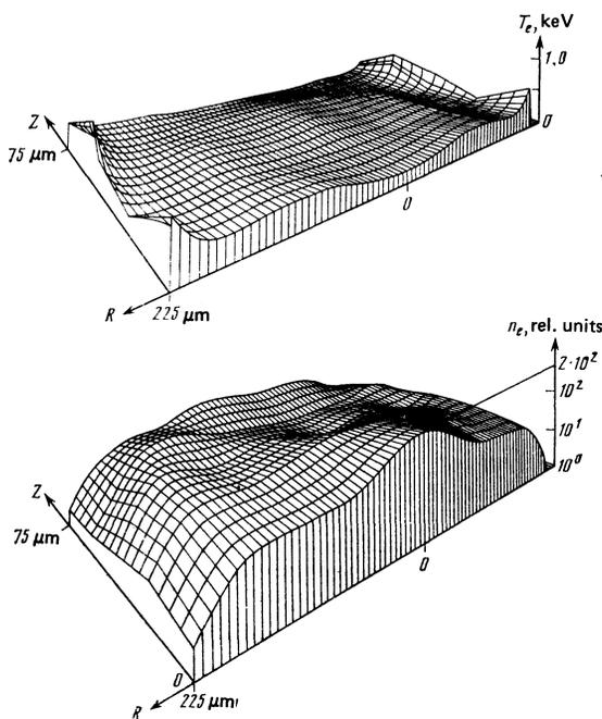
FIG. 1. Distributions of temperature and density constructed with automated processing of pin-hole-camera photographs by computer (aluminum target,  $E = 100$  J,  $\tau = 3.0$  nsec).
