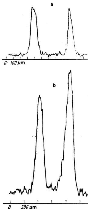
FIG. 5. Densitometer traces characterizing the distributions of intensity of the laser radiation at the focal spot (a) and sources of x radiation in the plasma corona (b) (aluminum target,  $E = 100 \text{ J}$ ,  $\tau = 3.0 \text{ nsec}$ ).
