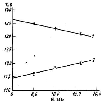
FIG. 8. Dependence on external magnetic field of the temperature of stability loss of axis:  $T_{\{100\}}$  (1) and  $T_{\{111\}}$  (2), for iron garnet  $Tb_{0.26}Y_{2.74}Fe_5O_{12}$ .
