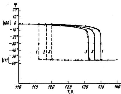
FIG. 7. Temperature dependence of the orientation of a single-crystal disk of  $Tb_{0.26}Y_{2.74}Fe_5O_{12}$  freely suspended in a magnetic field. The solid lines correspond to raising and the dashed to lowering of the temperature: 1,  $H = 5.0$  kOe; 2,  $H = 10.0$  kOe; 3,  $H = 16.1$  kOe.
