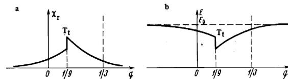
FIG. 3. Dependence of initial susceptibility (a) and Young's modulus (b) of a cubic ferromagnet on  $q = K_1/|K_2|$ .  $T_t$  is the temperature of the spin-reorientation phase transition.
