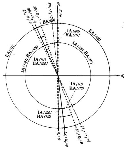
FIG. 1. Phase diagram of a single-domain cubic ferromagnet in zero magnetic field. Solid lines are phase-transition lines. Dashed lines are lines of interchange of the intermediate (IA) and hardest (HA) axes. Plotted with crosses are the lines of stability loss of the corresponding magnetic phases.
