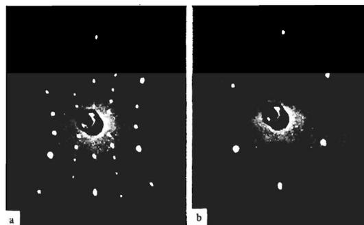
FIG. 1. Electron-diffraction patterns of the system Li-W (011): a—directly after annealing of film,  $(2 \times 3)$  structure; b—disappearance of superstructure reflections after electron bombardment of the surface.  $E = 55$  eV, current density  $j \approx 5 \times 10^{-4} \text{ A/cm}^2$ ,  $t = 13$  min,  $T = 5 \text{ K}$ .
