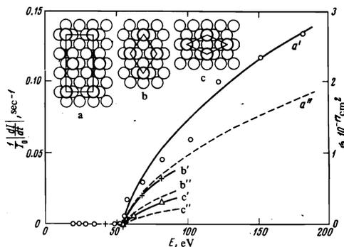
FIG. 3. Models a, b, and c—unit cells of the structures (2 X 3), c(2 X 2), and c(3 X 1) of lithium atoms on W(011); a', b', c'—dependence of initial rate of falloff of intensity I of reflections of structures a, b, and c on beam energy (left scale,  $I_0$  is the intensity at  $t = 0$ ); a'', b'', c''—dependence of cross section  $\sigma$  for structures a, b, and c on beam energy (right scale).
