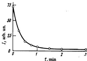
FIG. 2. Time dependence of the intensity of reflections of the (2 X 3) structure during electron bombardment of the surface.  $E = 80$  eV,  $T = 5$  K.
