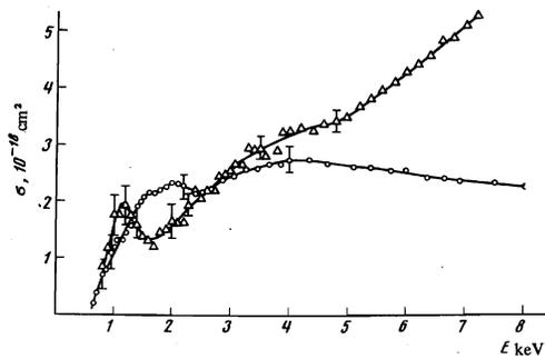
FIG. 4. Dependence of the excitation cross section of the NeII  $\lambda 326.1 \text{ \AA}$  line and of the resonance line NaII  $\lambda 376.4 \text{ \AA}$  on the energy of the  $\text{Na}^+$  ions.  $\Delta$ —excitation cross section of NaII  $\lambda 376.4 \text{ \AA}$  line,  $\circ$ —excitation cross section of the NeII  $\lambda 326.1 \text{ \AA}$  line.
