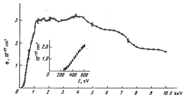
FIG. 3. Cross section for the excitation of the NeII  $\lambda$ 407.1 Å line vs. the energy of the  $\text{Na}^+$  ion. The insert shows the absolute radiation flux of all the lines whose wavelengths are shorter than  $\lambda_b = 575$  Å.
