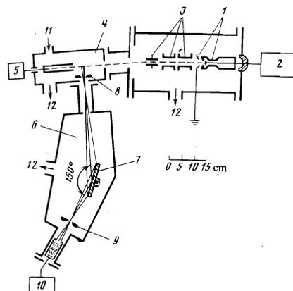
FIG. 1. Experimental setup: 1—ion source, 2—high voltage supply of ion source, 3—system for focusing the ion beam (quadrupole lens and clearing capacitor), 4—collision chamber, 5—ion receiver and ion-current recorder, 6—vacuum monochromator, 7—concave diffraction grating, 8, 9—entrance (stationary) and exit (movable) slits of the vacuum monochromator, 10—open electron multiplier and recording apparatus, 1—gas inlet, 12—to vacuum pump.
