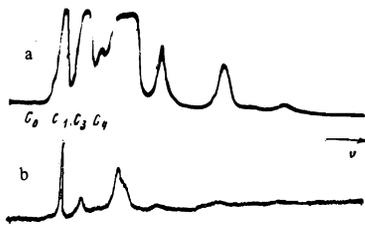
FIG. 1. Density patterns of the absorption spectrum of RbMnF<sub>3</sub> in the region of the  ${}^6A_{1g}({}^6S) \rightarrow {}^4E_g, {}^4A_{1g}({}^4G)$  transition at  $T = 20.4^\circ\text{K}$ : a—sample thickness 1.08 mm, b—normally exposed spectrum of sample 0.03 mm thick, which gives a qualitative idea of the intensity ratio of the fundamental absorption bands. Certain distinctly appearing bands are marked in accordance with the system adopted in Fig. 3 below.
