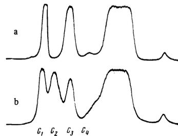
FIG. 2. Density patterns of the considered region of the RbMnF<sub>3</sub> spectrum at  $T = 20.4^\circ\text{K}$ . Sample thickness 0.8 mm. The spectra were obtained in unpolarized light with a certain prior exposition in order to reveal the details more clearly. a)  $H = 0$ , b)  $H = 300 \text{ kOe}$ .
