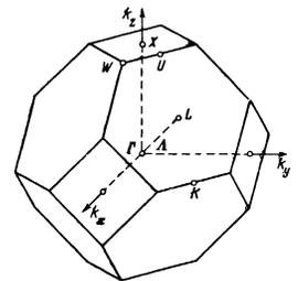
FIG. 4. Brillouin zone of antiferromagnetic RbMnF<sub>3</sub>.
