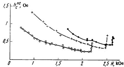
FIG. 5. Critical field  $h_C^{ne}$  against the static magnetic field at different temperatures: ●— $1.25^\circ\text{K}$ , ○— $1.55^\circ\text{K}$ , +— $1.7^\circ\text{K}$ .
