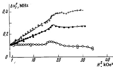
FIG. 8. Dependence of the relaxation  $\Delta\nu_2^e$  on the square of the static field  $H^2$  at different temperatures:  $\circ$  - 1.25°K,  $\bullet$  - 1.55°K,  $+$  - 1.70°K.
