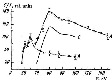
FIG. 3. Experimental excitation curves for the Ar II  $\lambda = 4880 \text{ \AA}$  line: the continuous curve A (with points) is the excitation curve obtained by modulating just the electron beam; the dashed curve B (with points) is the excitation curve obtained by simultaneous modulation of both beams; the continuous curve C is the difference between the other two curves, which is identical with the excitation function of the corresponding Ar II line in accordance with the reaction (4). [7]
