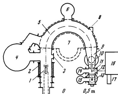
FIG. 1. Schematic diagram of the apparatus. 1—ion source 2—solenoid; 3, 8—viewing windows 4, 6, 10, 13, 14, 15—high-vacuum pumping units; 5—mass-spectrometer vacuum chamber; 7—mass-spectrometer magnet; 9—special high-vacuum chamber; 11—collision chamber 12—window for extraction of radiation; 16—spectroscopic instrument; 17—radiation (photon) detector.
