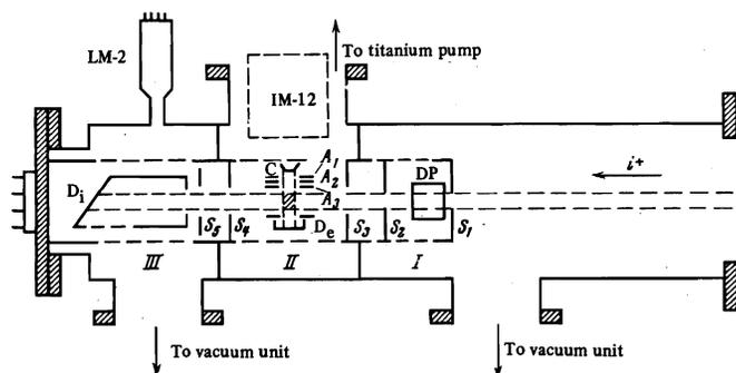
FIG. 2. Schematic diagram of the special high-vacuum chamber: 1–III—sections of the vacuum chambers;  $S_1$ – $S_4$  are slits; DP are deflecting plates; C is the electron gun cathode;  $A_1$ – $A_3$  are control electrodes in the electron gun;  $D_e$  and  $D_i$  are electron and ion detectors;  $S_5$  is an electrode for retardation of secondary electrons; IM-12 are LM-2 vacuum gauges.
