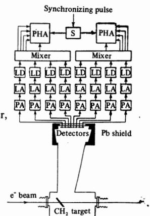
FIG. 1. Experimental apparatus: PA—pre-amplifier, LA—linear amplifier, LD—linear discriminator, S—shaper, PHA—pulse height analyzer.
