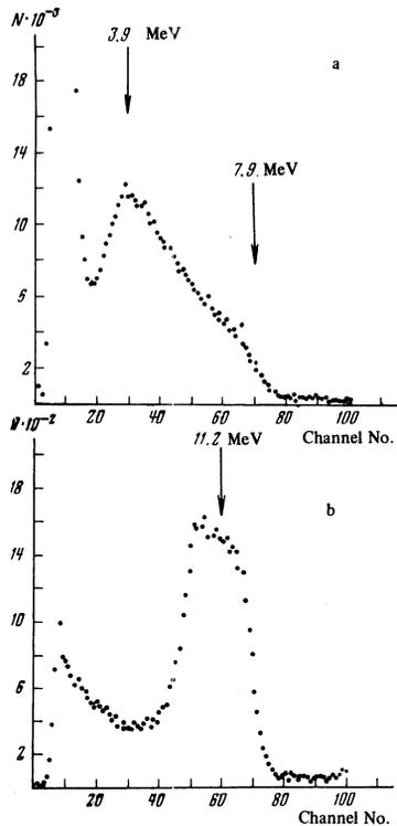
FIG. 2. Recoil-proton spectrum from  $\text{CH}_2$  target for two detectors: a— $40 \times 5 \times 0.7$  mm, b— $15 \times 15 \times 1$  mm.
