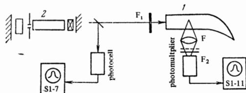
FIG. 4. Experimental setup. 1—Wood's horn with saturated rubidium vapor; 2—Q-switched ruby laser;  $F_1$ —calibrated neutral density filters;  $F_2$ —neutral density platinum filters; F—FS-7 optical filter.
