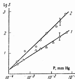
FIG. 5. Relative resonance fluorescence signal  $S$  as a function of molecular rubidium vapor pressure  $P$ : 1—weak excitation; 2—strong excitation.
