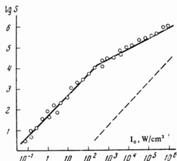
FIG. 3. Resonance fluorescence intensity  $S$  of  $\text{Rb}_2$  vapor as a function of single pulse intensity  $I_0$  of ruby laser.
