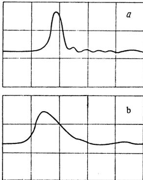
FIG. 6. Oscillograms of the exciting ruby laser pulse (a) and fluorescence pulse (b). Scale 20 nsec/division.
