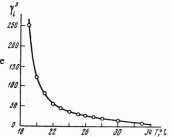
FIG. 4. Temperature dependence of the Grüneisen constant  $2\gamma_i^3$  for monocrystalline SbSI.
