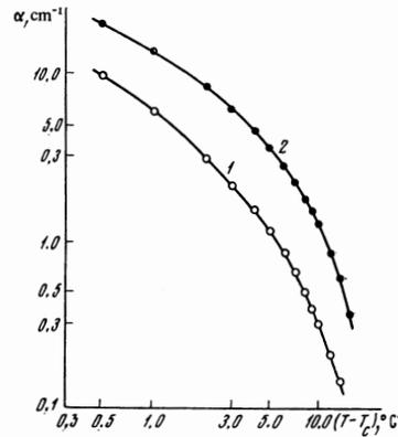
FIG. 3. Temperature dependence of the coefficients  $\alpha_1$  and  $\alpha_2$  of longitudinal USW. USW frequency: 1—15 MHz, 2—30 MHz.
