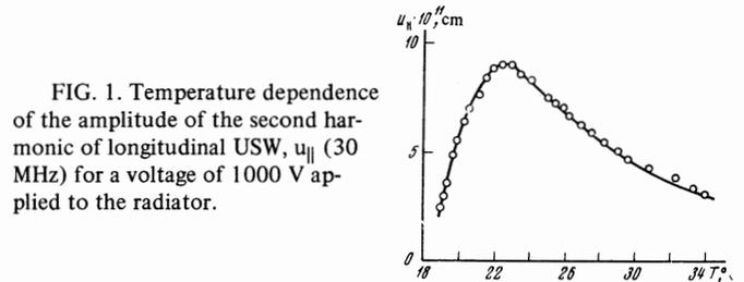
FIG. 1. Temperature dependence of the amplitude of the second harmonic of longitudinal USW,  $u_{||}$  (30 MHz) for a voltage of 1000 V applied to the radiator.
