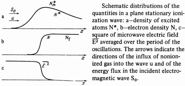
Schematic distributions of the quantities in a plane stationary ionization wave: a—density of excited atoms  $N^*$ , b—electron density  $N$ , c—square of microwave electric field  $\overline{E^2}$  averaged over the period of the oscillations. The arrows indicate the directions of the influx of nonionized gas into the wave  $u$  and of the energy flux in the incident electromagnetic wave  $S_0$ .
