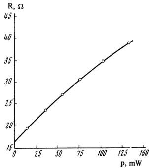
FIG. 3. Dependence of the resistance of the sample on the dc power absorbed in it.
