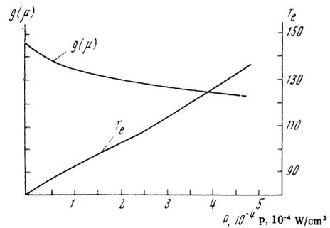
FIG. 1. Theoretical dependences of  $g(\mu)$  and  $T_e$  on the power absorbed per unit volume. The value of  $g(\mu)$  decreases from 0.75 to 0.7 when the temperature  $T_e$  increases from 77 to 140°K.
