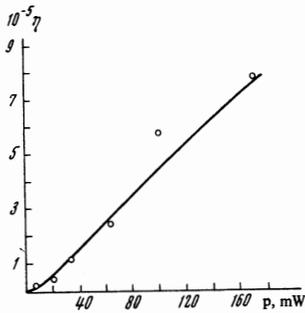
FIG. 5. Dependence of conversion coefficient  $\eta$  on the pumping power absorbed in the sample: the continuous curve is theoretical and the experimental points are denoted by  $\circ$ .
