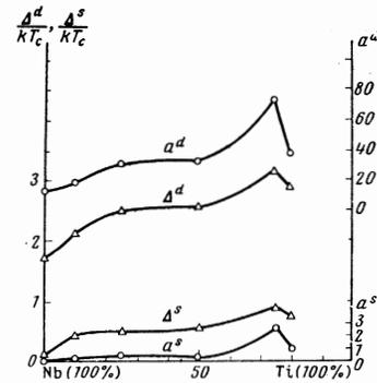
FIG. 3. Behavior of energy gaps  $\Delta^d/kT_c$  and  $\Delta^s/kT_c$  and of the pre-exponential factors  $a^d$  and  $a^s$  as functions of the concentration of titanium in the solid solution;  $\Delta^d$  and  $\Delta^s$ —behavior of the energy gaps of the d- and s-bands (in relative units) as functions of the titanium concentration;  $a^d$  and  $a^s$ —behavior of the pre-exponential factors for the d- and s-bands as functions of the titanium concentration.
