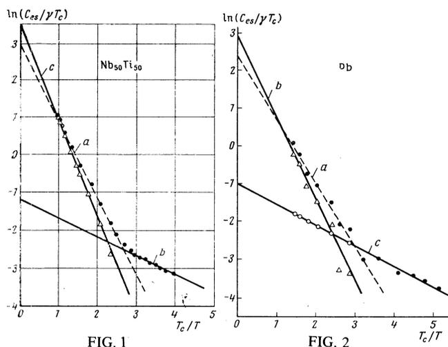
FIG. 1. Behavior of the specific heat of a sample 50% Nb + 50% Ti as a function of  $\ln C_{es}(T)/\gamma T_C$  vs.  $T_C/T$ . ●—experimental values; Δ—specific heat from the d-band (the specific heat of the s-band is subtracted); a—the slope of the dashed line determines the gap of the d-band, if no account is taken of the specific heat of the s-band; b—the slope of this straight line determines the gap of the s-band; c—the slope of the solid line gives a more accurate value of the d-band gap.
