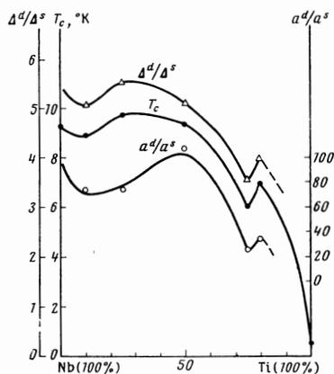
FIG. 4. Concentration dependence of the ratio of the energy gaps of the d- and s-bands,  $\Delta^d/\Delta^s$ , of the transition temperature  $T_c$ , and of the ratio  $a^d/a^s$  of the pre-exponential factors.
