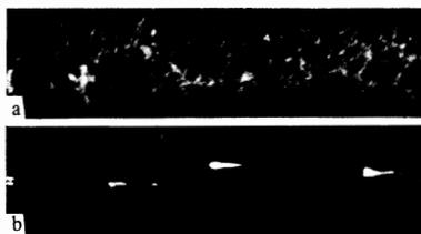
FIG. 4. Damage in LiNbO<sub>3</sub> crystals at 1.06  $\mu$ . a—Sample No. 1 (with scattering centers). The damage has the form of a track consisting of microcracks. Magnification 58 times. b—pure Sample No. 2. Damage in the form of a long thread. Magnification 30 times.
