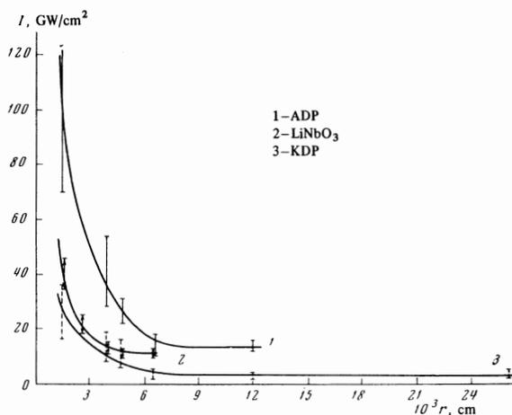
FIG. 5. Dependence of damage threshold on focal length of lens (focal radius of laser beam) at  $1.06 \mu$ .
