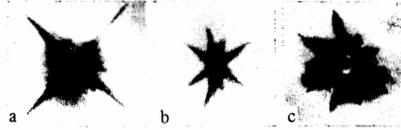
FIG. 2. Characteristic damage of KDP and ADP crystals. Magnification 34 times. a—cracks along  $\{110\}$  planes; b—cracks along  $\{012\}$  planes and two cracks close to  $\{001\}$ ; c—opaque nucleus frequently observed in the center of the damaged spot.
