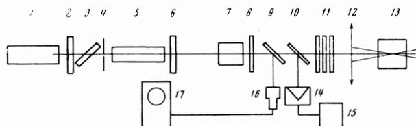
FIG. 1. Block diagram of the experimental arrangement: 1—gas laser ( $\lambda = 6328 \text{ \AA}$ ); 2, 6—dielectric mirrors; 3—passive shutter; 4—diaphragm, 1.5 to 2 mm; 5—neodymium-glass rod, 8 mm diameter, length 130 mm (glass LGS-5); 7—KDP frequency doubler ( $\varphi = 0^\circ$ ,  $\theta = 57^\circ$ ); 8—SZS-21 filter; 9, 10—plane-parallel glass plates; 11—neutral filters; 12—spherical lens; 13—sample; 14, 15—calorimeter; 16—FÉK-09 photoelement; 17—S1-11 oscilloscope.
