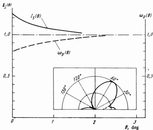
FIG. 3. Angular dependence of the intensity of scattering by a transverse polariton in a GaP crystal in the region of small  $\theta$ . The frequency unit is  $\omega_f = 367 \text{ cm}^{-1}$ . In the right-hand corner we show schematically the scattering indicatrix.
