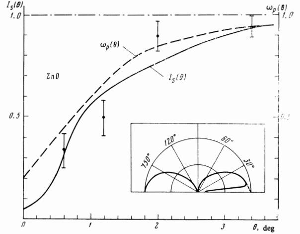
FIG. 4.  $I_S(\theta)$  plot for scattering in ZnO crystal ( $\omega_f = 407 \text{ cm}^{-1}$ ) in the region of small  $\theta$ . The scattering indicatrix is shown schematically in the right-hand corner. Points – values of  $I_S(\theta)$  in accordance with the spectrograms from [4].
