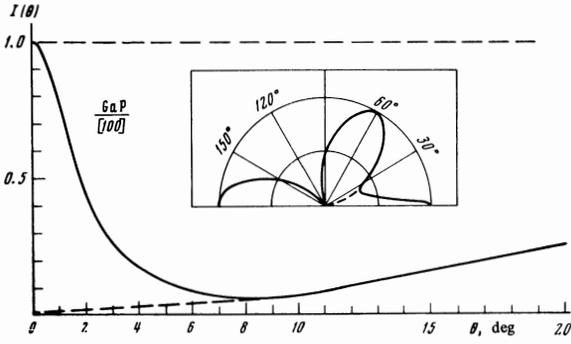
FIG. 2. Angular dependence of the intensity of scattering by a longitudinal phonon ( $\omega_f = 404 \text{ cm}^{-1}$ ) in a GaP crystal.
