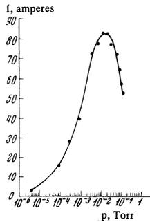
FIG. 2. Pressure dependence of electron emission current.
