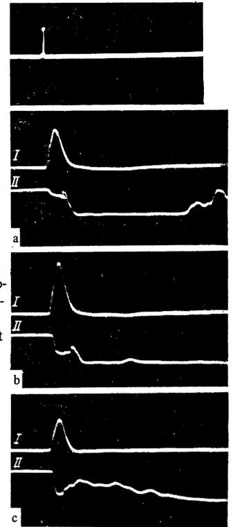
FIG. 3. Oscillograms of the electron emission current I and the microwave cutoff signal II at different pressures. The oscillogram at the top represents the registration of a laser light pulse.  $p =$  (a)  $10^{-3}$ , (b)  $2 \times 10^{-2}$ , and (c)  $10^{-1}$  Torr.
