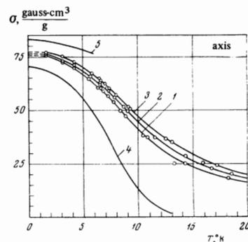
FIG. 2. Temperature dependence of  $\text{Eu}_3\text{O}_4$  magnetization along the  $c$  axis in different magnetizing fields:  $H_e =$  (1) 13.94 kOe, (2) 16 kOe, (3) 17.16 kOe, (4) 0, (5)  $\infty$ .
