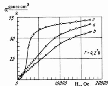
FIG. 1. Magnetization curves of  $\text{Eu}_3\text{O}_4$  along three perpendicular axes.
