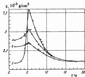
FIG. 4. Temperature dependence of  $\text{Eu}_3\text{O}_4$  susceptibility along the different axes for  $H_e = 1.2 \text{ kOe}$ .
