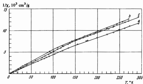
FIG. 5. Temperature dependence of inverse susceptibility along different  $\text{Eu}_3\text{O}_4$  axes.
