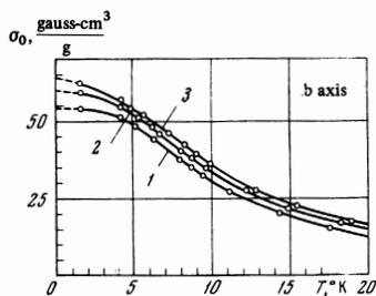
FIG. 3. Temperature dependence of  $\text{Eu}_3\text{O}_4$  magnetization along the b axis in three different magnetizing fields: (1) 13.94 kOe, (2) 16 kOe, (3) 17.16 kOe.
