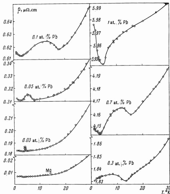
FIG. 2. Temperature dependence of the resistivity of pure Mg and of Mg - Pb alloys.
