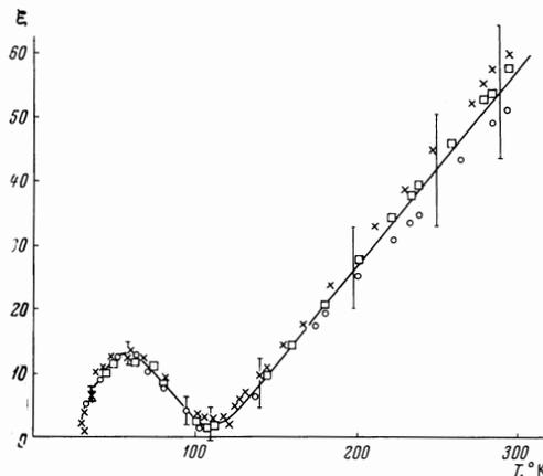
FIG. 3. Temperature dependence of the relative change in the resistivity  $\xi = [\Delta\rho(T) - \Delta\rho(0)]/c\rho_{Mg}(273^\circ)$  for Mg - Pb alloys: X - 0.1 at.% Pb, □ - 0.05 at.% Pb, ○ - 0.03 at.% Pb.
