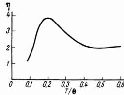
FIG. 5. Calculated temperature dependence of the relative change in the electrical resistivity of a Mg–Pb alloy;  $\eta = [\Delta\rho(T) - \Delta\rho(0)]/c\rho_{\text{Mg}}(2\Theta/3)$ .
