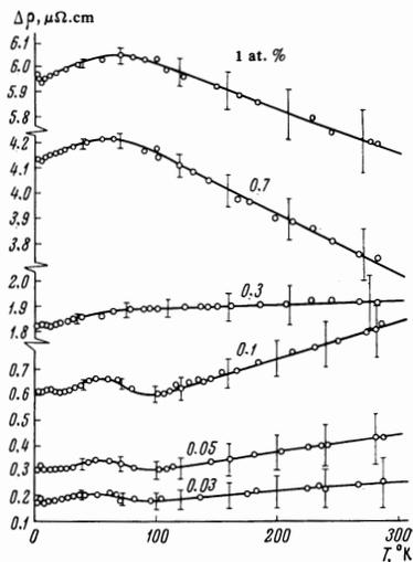
FIG. 1. Temperature dependence of the impurity resistivity of Mg - Pb alloys with various concentrations of Pb.
