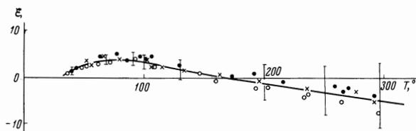
FIG. 4. Temperature dependence in the relative change in the resistivity of Mg - Ag alloys: ○ - 0.3 at.% Ag, X - 0.05 at.% Ag, ○ - 0.03 at.% Ag.
