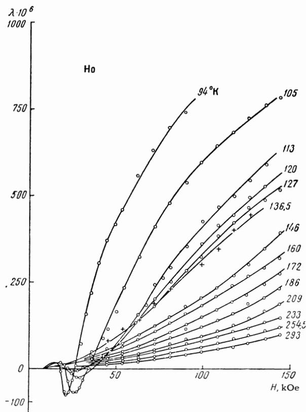
FIG. 3. Dependence of magnetostriction on field at constant temperature in Ho.
