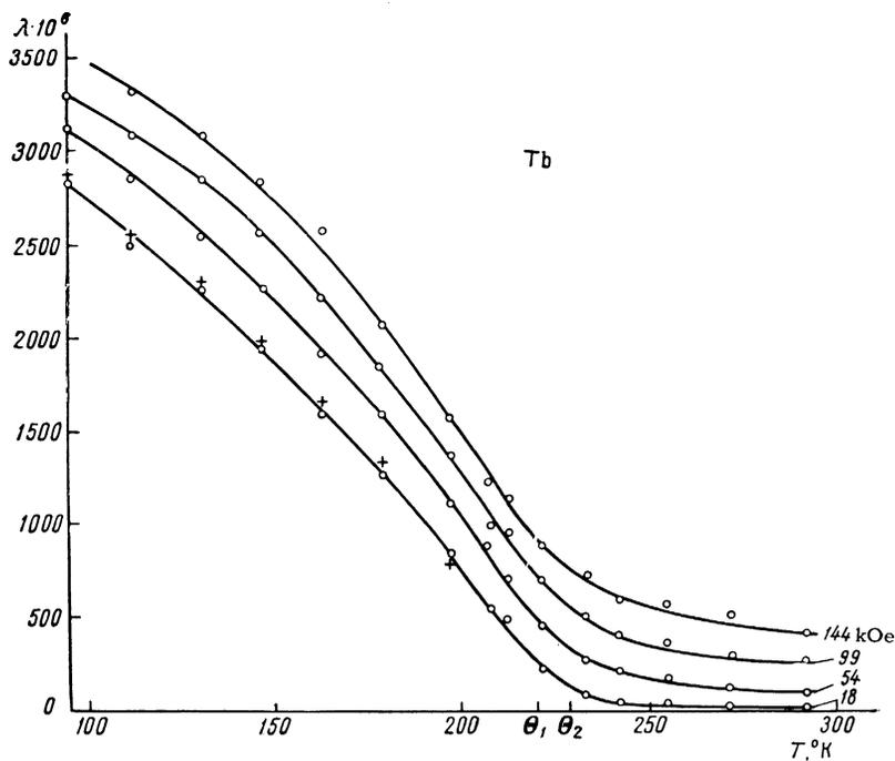
FIG. 5. Dependence of magnetostriction on temperature at constant field in Tb; +, dependence of  $\lambda_s(T)$ .
