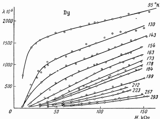
FIG. 2. Dependence of magnetostriction on field at constant temperature in Dy.
