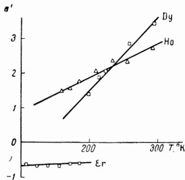
FIG. 9. Dependence of the coefficient  $a'$  (in  $10^{-8} \text{ Oe}^{-2}$ ) on temperature.
