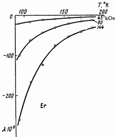
FIG. 8. Dependence of magnetostriction on temperature at constant field in Er.
