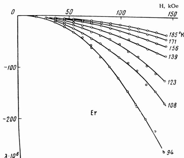
FIG. 4. Dependence of magnetostriction on field at constant temperature in Er.
