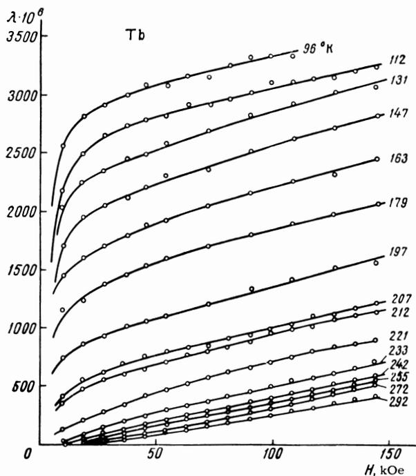
FIG. 1. Dependence of magnetostriction on field at constant temperature in Tb.
