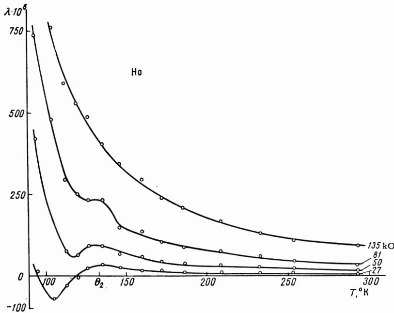
FIG. 7. Dependence of magnetostriction on temperature at constant field in Ho.
