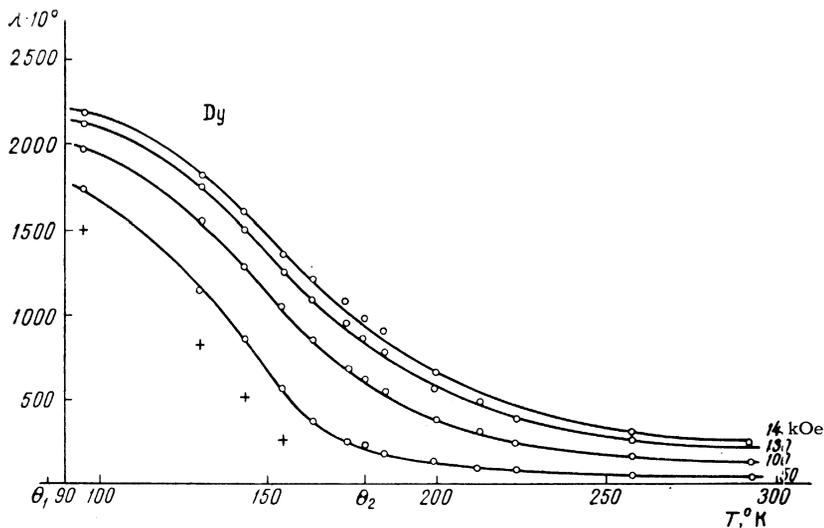
FIG. 6. Dependence of magnetostriction on temperature at constant field in Dy; +, dependence of  $\lambda_s(T)$ .
