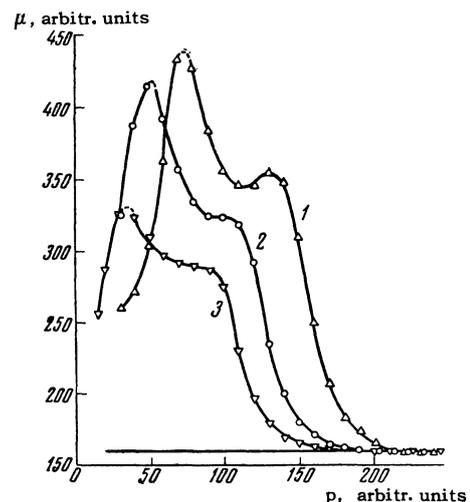
FIG. 2. Dependence of the permeability of alloy No. 1 on pressure at various temperatures: 1) at  $0^\circ\text{C}$ ; 2)  $+13.5^\circ\text{C}$ . 3)  $+19.5^\circ\text{C}$ .
