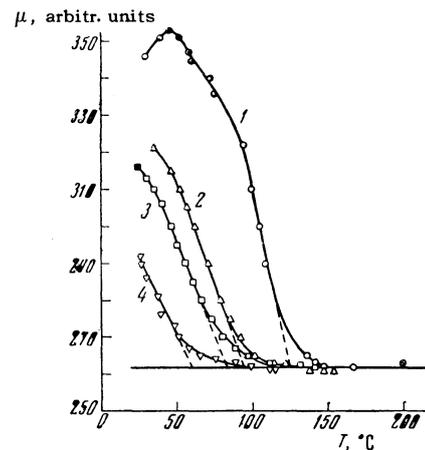
FIG. 1. Dependence of the permeability of alloy No. 2 on temperature at various pressures: 1)  $p = 0.3$  kbar,  $\Theta = 125^\circ\text{C}$ ; 2)  $p = 3.7$  kbar,  $\Theta = 95^\circ\text{C}$ ; 3)  $p = 5.9$  kbar,  $\Theta = 83^\circ\text{C}$ ;  $p = 8.1$  kbar,  $\Theta = 60^\circ\text{C}$ .
