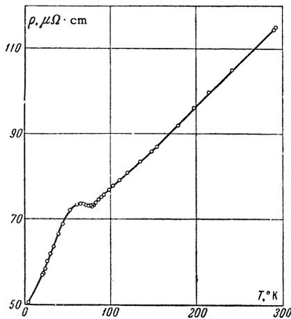
FIG. 5. Dependence of the electrical resistivity of Er on temperature.
