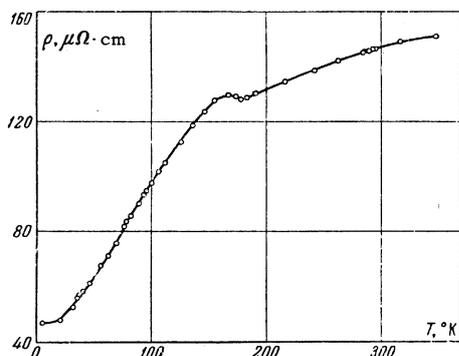
FIG. 2. Dependence of the electrical resistivity of Dy on temperature.
