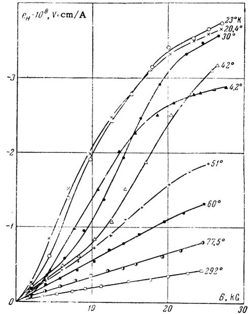
FIG. 6. Dependence of the specific Hall emf of Er on the magnetic induction at certain characteristic test temperatures.
