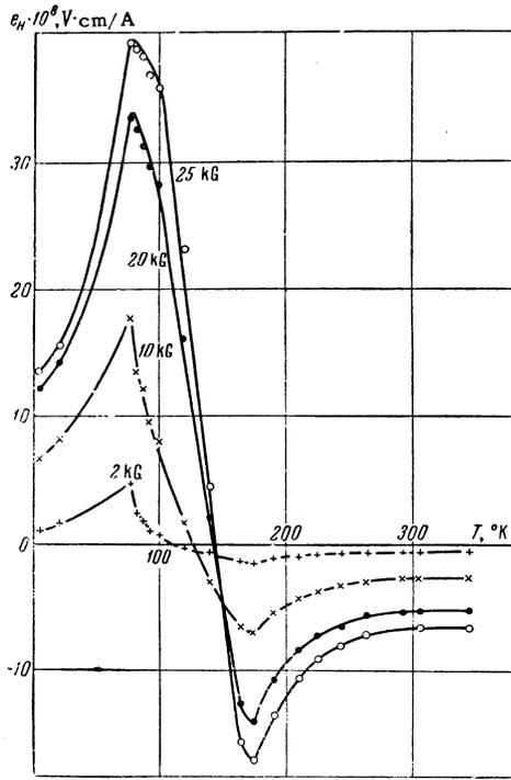
FIG. 4. Dependence of the specific Hall emf of Dy on temperature at various values of the magnetic induction in the sample.
