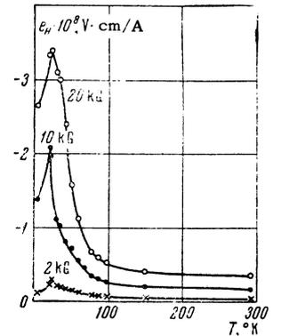
FIG. 7. Dependence of the specific Hall emf of Er on temperature at various values of the magnetic induction in the sample.
