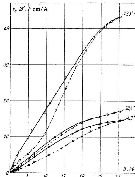
FIG. 3. Dependence of the specific Hall emf of Dy on the magnetic induction in the ferromagnetic region.
