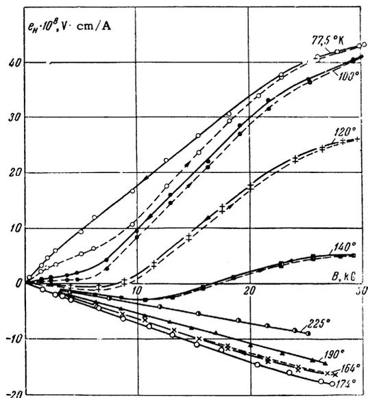
FIG. 1. Dependence of the specific Hall emf ( $e_H = Ed/I$ ) of Dy on the magnetic induction at certain characteristic test temperatures.
