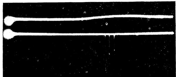
FIG. 3. Emission of an optical generator with modulated  $Q$ . Length of scan—100  $\mu$ sec. The second trace records the approximate position of the aperture at the moment of pulse generation.
