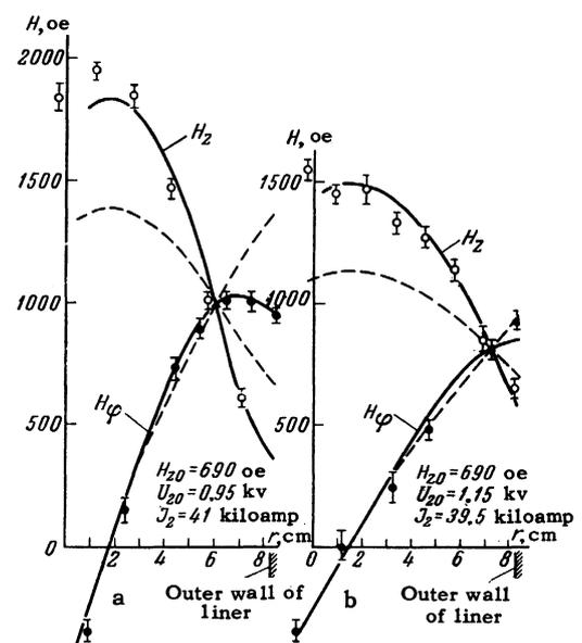
FIG. 1. Distribution of the longitudinal ( $H_z$ ) and azimuthal ( $H_\phi$ ) components of the magnetic field in the discharge: a - thick-wall aluminum liner; b - thin-wall liner made of nonmagnetic steel. Solid curves - force-free model, dashed - paramagnetic model.
