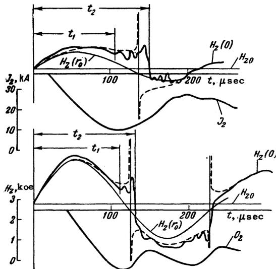
FIG. 2. Oscillograms of discharge current  $J_z$  and longitudinal magnetic field  $H_z(0)$  at the center of the chamber upon application of an alternating magnetic field ( $r_0$  – radius of liner). The dashed curve is calculated in force-free model.
