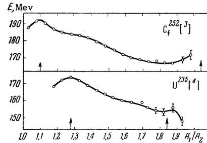
FIG. 2. Change in the total kinetic energy as a function of the ratio of the fragment masses. The curves were plotted from the experimental data of Fraser and Milton<sup>3</sup> and Stein.<sup>4</sup> The positions of the "magic" fragments are indicated by arrows.
