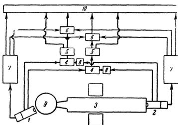
FIG. 1. Schematic diagram of experimental setup. 1, 2) photomultipliers, 3) magnetic lens spectrometer, 4) fast-coincidence circuits, 5) amplifiers, 6) slow-coincidence circuits, 7) pulse-height analyzers, 8) variable-delay lines, 9) sample under study, 10) scaler circuit and electromechanical counters.
