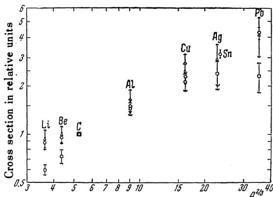
FIG. 2. Dependence of  $\pi$ -meson yield on atomic weight.  $\circ$  —  $\pi^0$  mesons,  $\Delta$  —  $\pi^-$  mesons,  $\square$  —  $\pi^+$  mesons.
