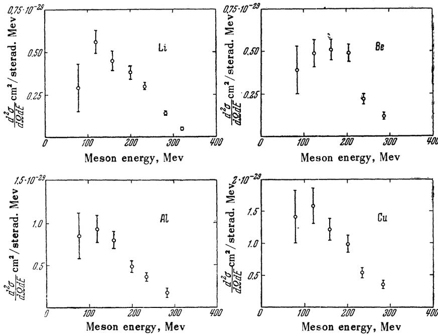
FIG. 1. Spectra of  $\pi^-$ -meson production
