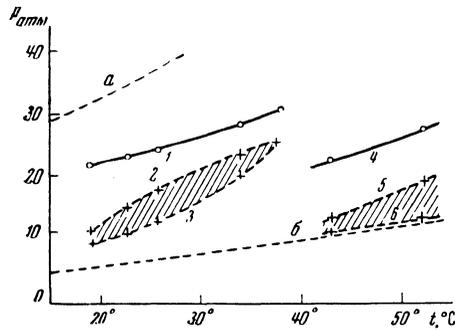
Dash lines — pressures of the unsaturated vapors of pure: (a) Freon-13, (b) Freon-12. Solid curves — same for the mixtures: (1) 40% Freon-12, (4) 75% Freon-12. Curves 2 and 3 bound the working region for the first mixture; curves 5 and 6 bound the region for the second mixture.
