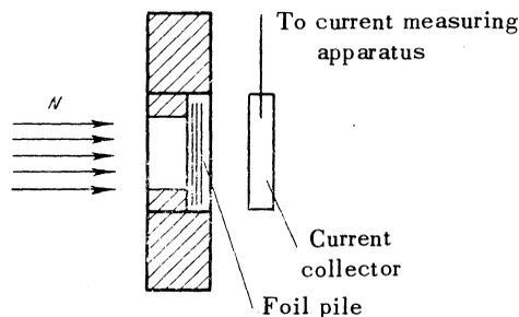
FIG. 1. Arrangement of the targets in the experiment
