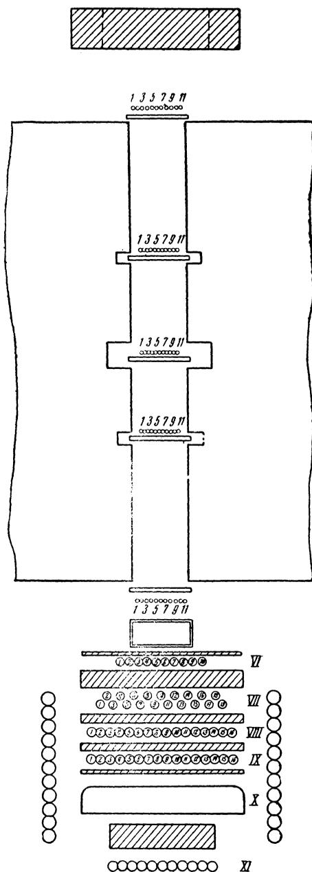
FIG. 1. Distribution of the counters in the telescope and of the absorbers.
