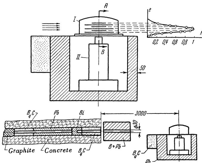
FIG. 1. I—Multifoil ionization chamber; II—Scintillation counter. Above on the right is given the distribution of neutron flux across the cut AB. The arrows on the left indicate the neutron direction of motion.
