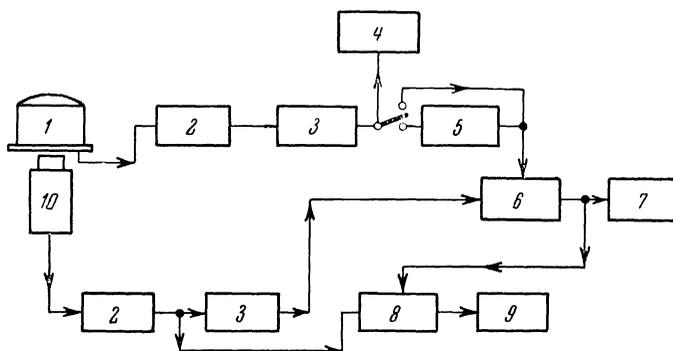
FIG. 2. Block Diagram of Electronics. 1—Ionization chamber, 2—Amplifier, 3—Discriminator, 4—Scalar ( $\times 10^4$ ), 5—Delayline, 6—Coincidence circuit, 7—Scalar ( $\times 64$ ), 8—Gate circuit, 9—20 channel analyzer. 10—Scintillation counter.
