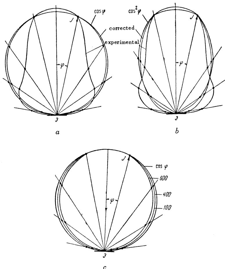
FIG. 4. Corrected angular distributions: *a.* assumed distribution  $\sim \cos \varphi$ ; *b.* assumed distribution  $\sim \cos^2 \varphi$  ( $V_p = 400$  v,  $V_k = 30$  v for both *a* and *b*); *c.* assumed distribution  $\sim \cos \varphi$ ,  $V_p = 100, 400$ , and  $600$  v.
