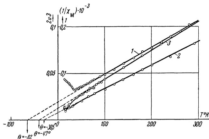
FIG. 4. Temperature dependence of the reciprocal of the molar magnetic susceptibility,  $1/\chi_M$  of anhydrous  $\text{CuSO}_4$ . The dotted curve was drawn according to formula (2).
