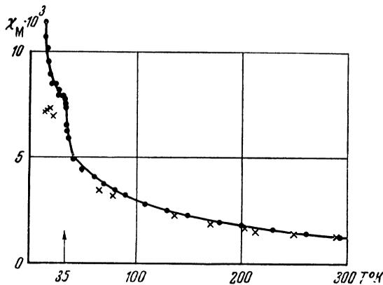
FIG. 2. Temperature dependence of the molar magnetic susceptibility  $\chi_M$  of anhydrous  $\text{CuSO}_4$ .  $\times$ , results of the Leiden laboratory<sup>11</sup>;  $\bullet$ , data from the present work.
