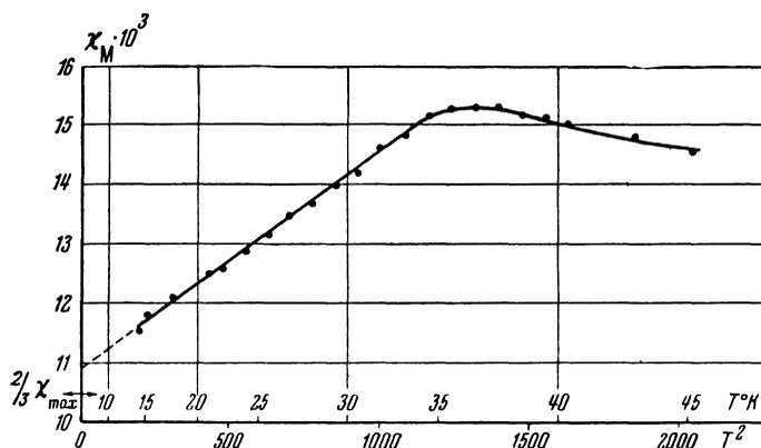
FIG. 5. Temperature dependence of the magnetic susceptibility of the anhydrous sulfate  $\text{NiSO}_4$  below the Curie point.
