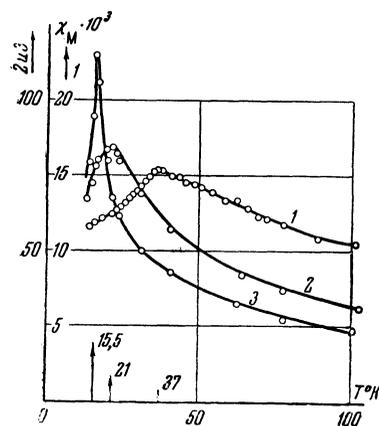
FIG. 1. Temperature dependence of the molar magnetic susceptibility  $\chi_M$  of anhydrous sulfates: 1,  $\text{NiSO}_4$ ; 2,  $\text{FeSO}_4$ ; 3,  $\text{CoSO}_4$ . The values of  $T_C$  are shown by the arrows.
