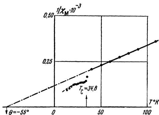
FIG. 3. Temperature dependence of the reciprocal of the molar magnetic susceptibility,  $1/\chi_M$ , of anhydrous CuSO<sub>4</sub>. The dotted curve was drawn according to the formula (2).
