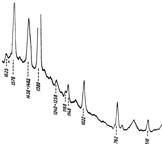
FIG. 1. Spectrum of combination scattering of powdery naphthalene. Voltage source FEU, 910 volts. The width of inlet and outlet slits was 0.2 mm. Frequencies (in  $\text{cm}^{-1}$ ) are shown for certain lines of combination scattering.
