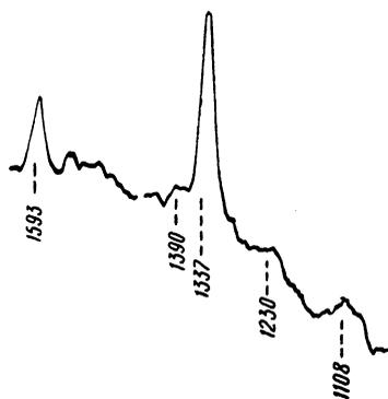
FIG. 2. Spectrum of combination scattering of powdery paranitrotoluene. Supply voltage FEU, 910 volts. Width of inlet slit, 0.7 mm, outlet slit, 0.2 mm. Frequencies (in  $\text{cm}^{-1}$ ) are shown for certain lines of combination scattering.
